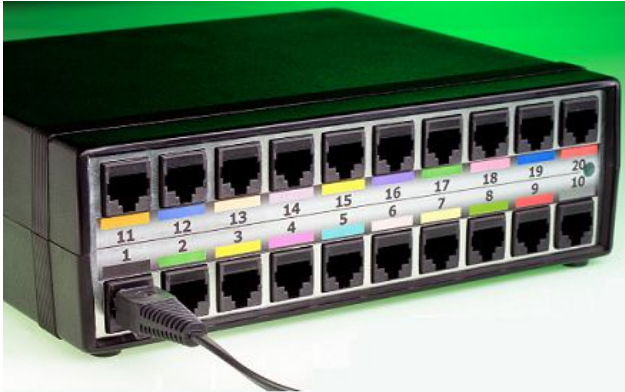
Figure 2 Front face of multiplexer box with RJ45 sensor ports.
