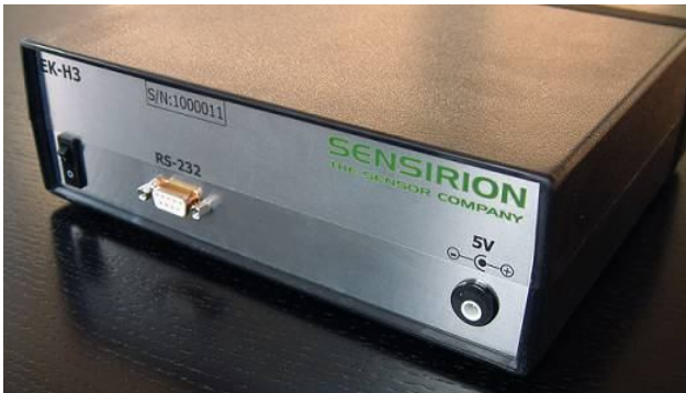
Figure 3 Rear face of the multiplexer box with RS-232 port to the computer in the middle/left and one port for power supply to the right. The on/off plug is located to the left.
